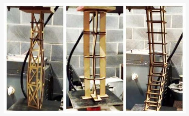
**Figure 10.** Photographs of laser cut model towers being load tested in Week 12 in the Civil Engineering Laboratory (from 2019/20)
